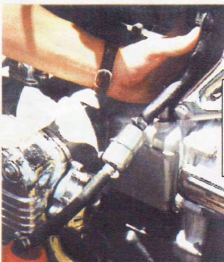
Figure 7-A Draining old fuel from tank
