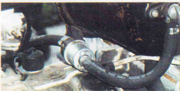
Figure 8-A Fuel filter mounted into position after lines are attached.
