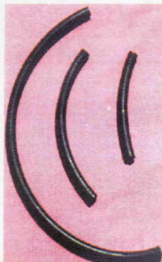
Figure 24-B three fuel lines 6", 9" and 21"
