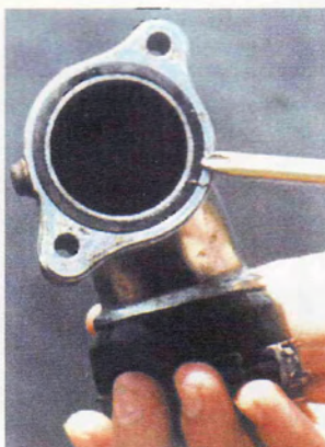
Figure 15-C o-ring in 90 deg. Intake fitting
