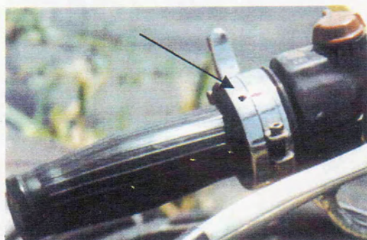
Figure 14A push and pull cables installed. Illustrated with throttle in full open position
