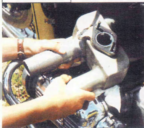
Figure 10-A Sliding new manifold into position
