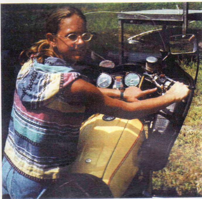
Figure 21-B recommended two hand starting procedure, to prevent flooding bike with accelerator pump
