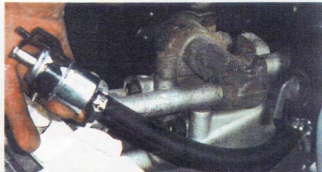
Figure 7-B Attaching fuel lines to filter before mounting the filter will make a trouble free installation
