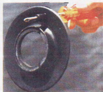
Figure 17-D air filter adapter ring with hold drilled out
