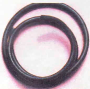
Figure 25-A vacuum line for GL1100
