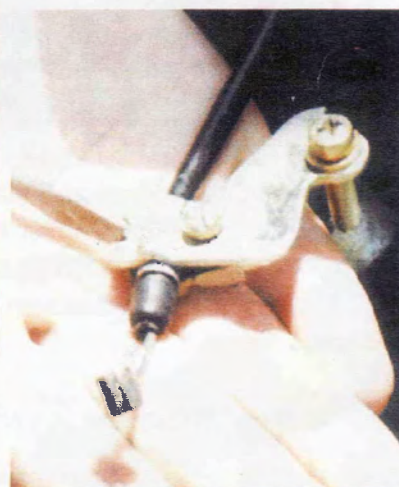
Figure 10-C choke cable bracket removed
