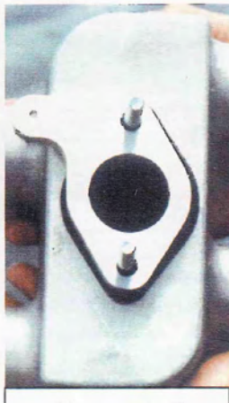
Figure 9-C Manifold with riser.
