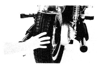
Loosely reinstall the left shock absorber bolt to support the swing arm.
