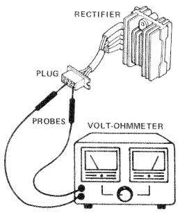
Check the silicon rectifier resistances with an ohmmeter.
