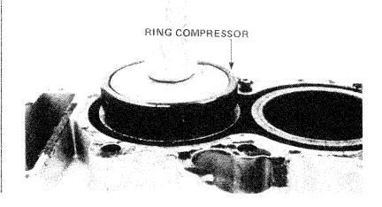
Install the left-hand rod assemblies for cylinders 2 and 4 with the rod oil holes facing the engine top.
