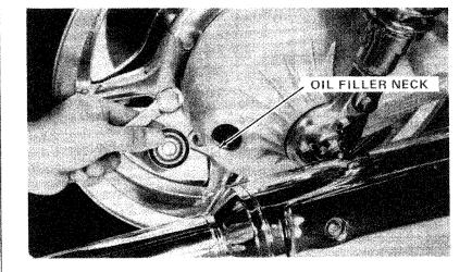
If the level is below the filler neck add the recommended lubricant until it reaches the filler neck threads. Reinstall the filler cap.
