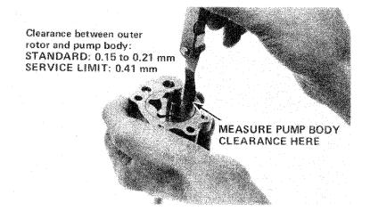
Measure pump end clearance. Lay straight edge on pump body.
