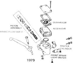
Place the master cylinder on the handlebar and install the holder and the two mounting bolts making sure that the high mating surface of the holder is on the top and the top bolt is tightened first. Install the brake line bolt and its two sealing washers. Install the brake lever and bolt and nut.
