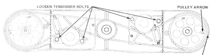
MOVE TENSIONER ROLLERS AWAY FROM BELTS AND RETIGHTEN BOLTS. Remove the belts.
