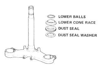
Grease the top race and install the 18 ball bearings. Grease the lower cone race and install the 19 ball bearings on the race.
