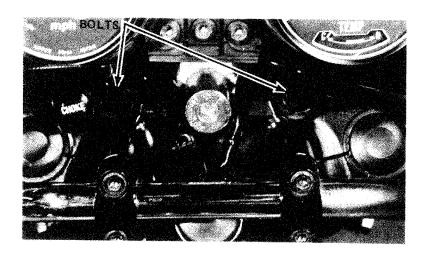
Remove the 2 ignition mounting bolts and ignition switch.
