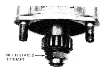
Secure the spline with the pinion holder HC 41305 and remove the nut and washer.
