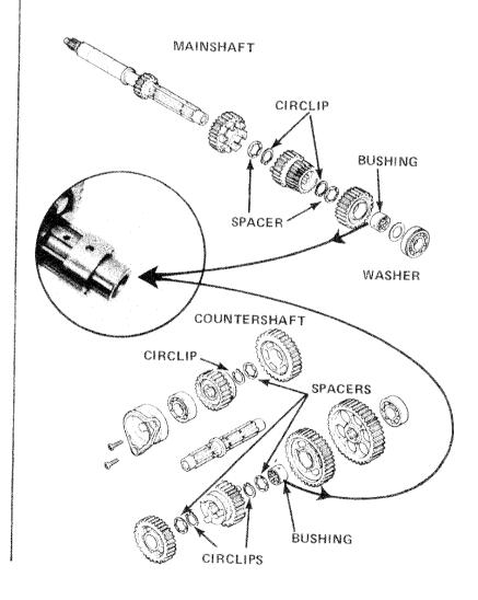
With the bearings firmly in place on the mainshaft, measure the assembled length to insure proper alignment with case bearing set rings.
