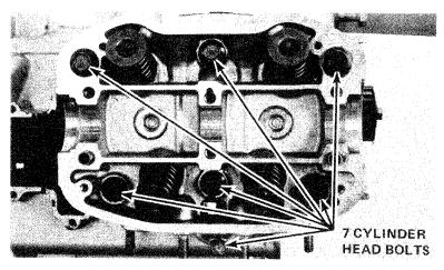
Support the intake manifold and remove cylinder head.
