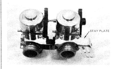
Separate each pair of carburetors at the throttle link and at the choke link. Be careful not to lose the spring placed between the throttle rods or the choke link connector.
