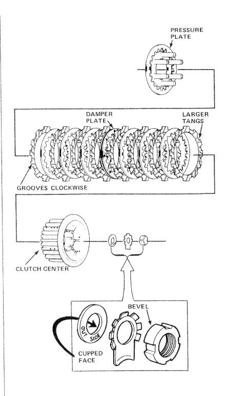
Torque the clutch center nut using the special clutch holder HC 41304 and socket wrench HC 41303 and bend up a lock tab.
