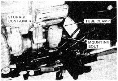
The storage container should be emptied every 6,000 kilometers (3,750 miles). More frequent service may be required if the motorcycle is operated in rainy weather or at full throttle. The section of drain tube just above the storage container is transparent, so the accumulated fluid will be visible if the container becomes overfilled.
