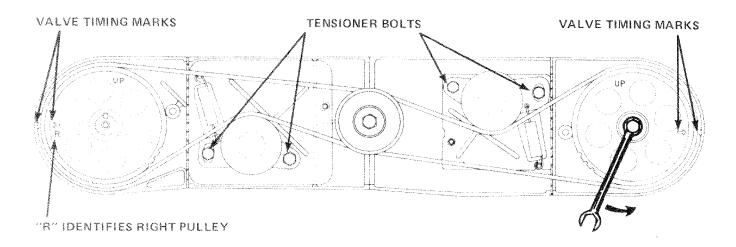
Apply pressure counter-clockwise on the camshaft pulley so the belt will be slack at the tensioner. With the tensioner bolts loosened, the spring pressure automatically positions the tensioner. Tighten the tensioner bolts. Recheck valve timing.
