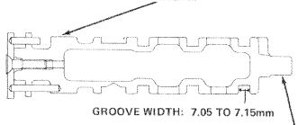
DRUM MINOR O.D.: 11.966 TO 11.984mm SERVICE LIMIT: 11.95mm
