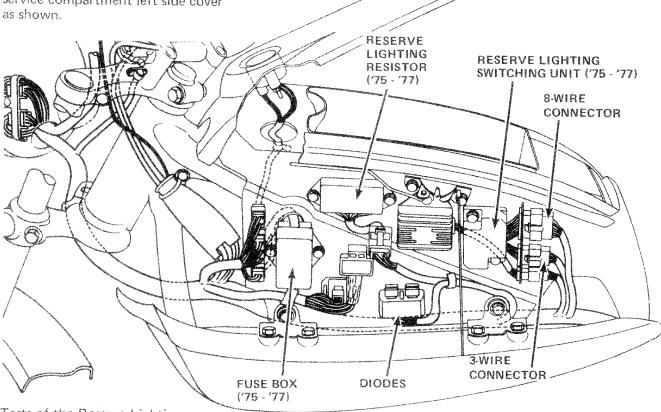
Tests of the Reserve Lighting System include input and output voltages and continuity tests of the resistor and two diodes.
