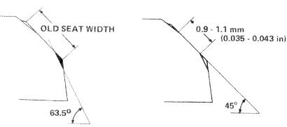
After cutting the seat, apply lapping compound to valve face, and lap the valve using light pressure.
