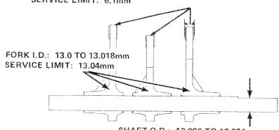
SHAFT O.D.: 12,966 TO 12,984mm SERVICE LIMIT: 12,90mm
