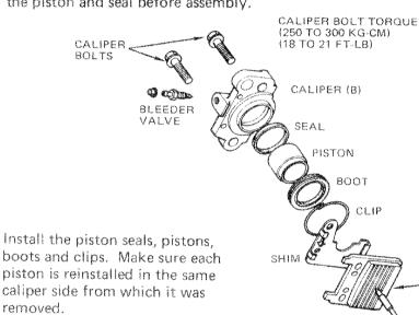
Install the shims, pads, pins and spring. The arrows on the shims must be pointing down when the caliper is positioned on the motorcycle. The seal between the two caliper halves should be replaced with a new seal.
