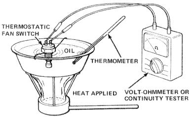
SWITCH OPEN (NO CONTINUITY) BELOW 93-97°C (199-207°F). SWITCH CLOSED (CONTINUITY) 98-102°C (208-215°F).
