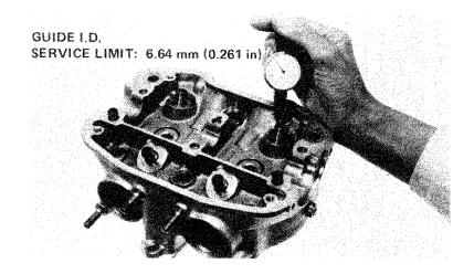
VALVE STEM-TO-GUIDE CLEARANCE SERVICE LIMITS
