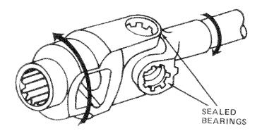
Clean the splines of the rear coupling and check the backlash.
