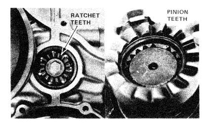
Straighten the lock tab. Remove the quide bolt, ratchet flange and quide plate.
