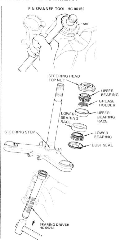
Remove the lower bearing outer race, using bearing driver HC 64768 and race removal tool HC 64766.
