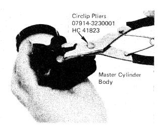
Remove the stop plate, secondary cup and piston. Then remove the primary cup, spring and check valve (1975 - 1977 models only require check valve removal).
