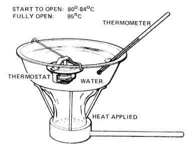
VALVE LIFT: 8 mm (0.32 in) MINIMUM WHEN HEATED TO 97°C FOR FIVE MINUTES.
