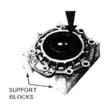
Inspect the 6914 bearing for smooth operation. If replacement is necessary, remove the bearing with a press.
